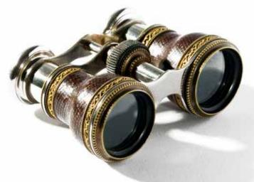
Following the invention of the telescope in the 17th century, the advantages of mounting two of them side by side for binocular vision became obvious. Developed by Italian optician, Ignazio Porro in 1854 and made popular by the Carl Zeiss Company in the 1890s, **Binoculars** give users a three-dimensional image, presented to each of the viewer's eyes from slightly different viewpoints. This merged view provides a greater impression of depth.
